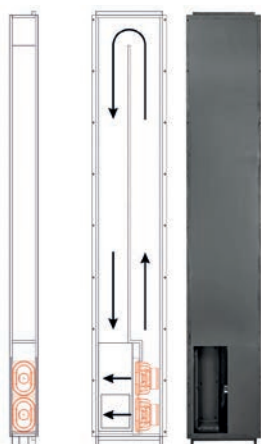
Wisdom's Regenerative Transmission Line (RTL) tech can generate 123dB at 20Hz from the twin 5x7-inch drivers inside the super-thin S90i in-wall design
