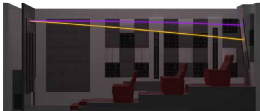
Power over distance: Line Sources have half the propagation loss of Point Sources, providing a better row to row consistency
