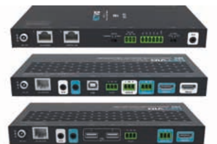
Netvio's new JP4 AVoIP platform will handle 4K/60 HDR over standard 1Gb IP and offers a real-time 1080p preview stream on Apple and Android devices
