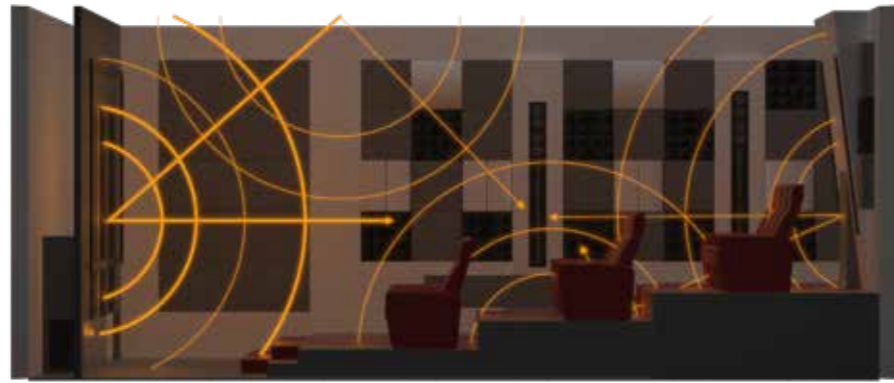
Point of confusion: Point Source propagates in all directions providing more reflected sound v direct sound
